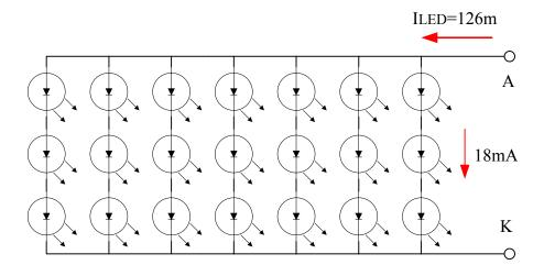
■ The constant current source is needed for white LED back-light driving. When LCM is operated over 60°C ambient temperature, the I<sub>LED</sub> of the LED back-light should be adjusted to 105mA max
