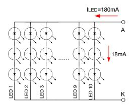
The constant current source is needed for white LED back-light driving. When LCM is operated over  $60^{\circ}$ C ambient temperature, the I<sub>BL</sub> of the LED back-light should be adjusted to 135mA max
