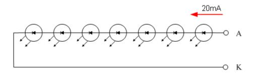
The constant current source is needed for white LED back-light driving.
