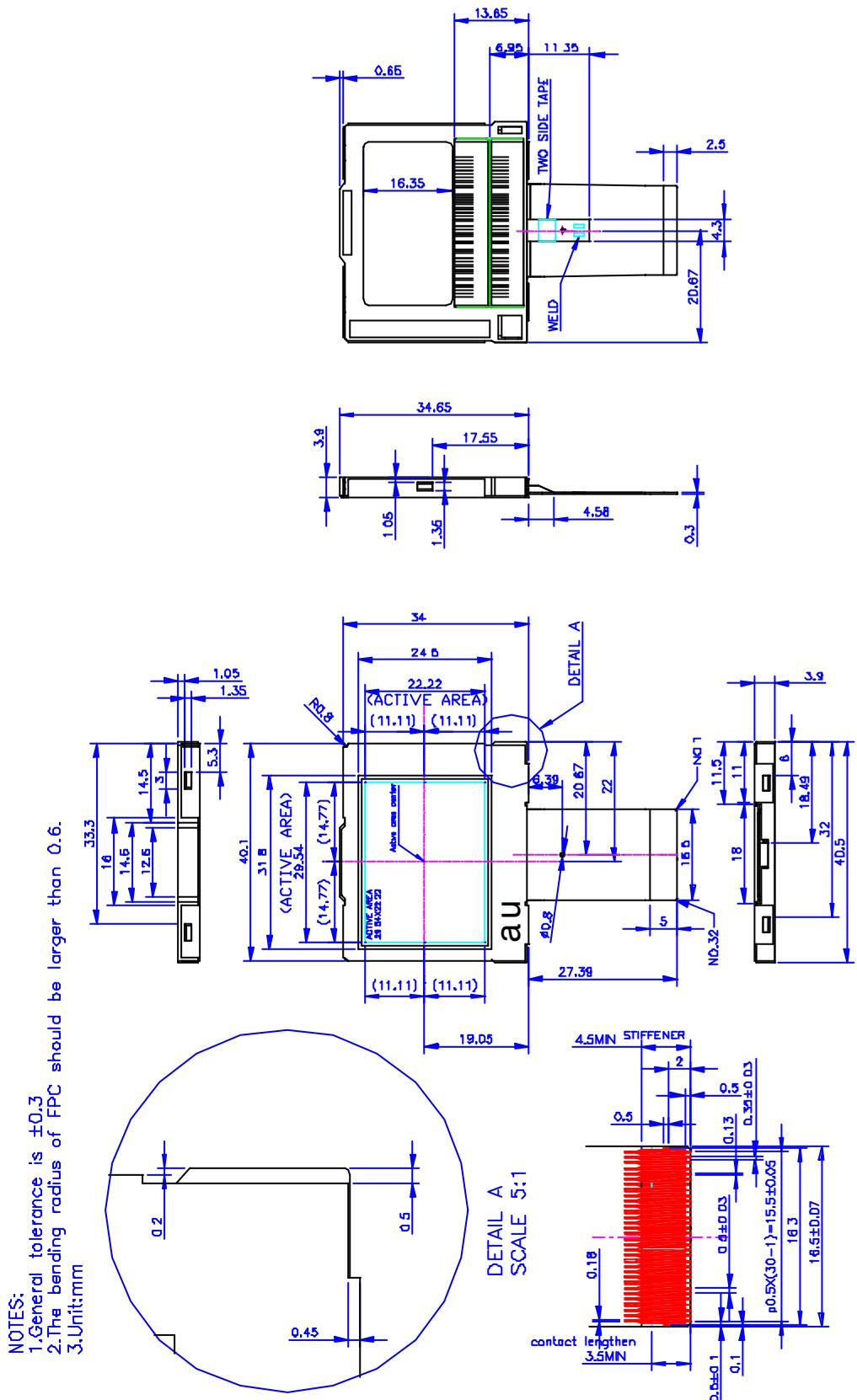
**Fig.4** Outline dimension of TFT-LCD module
