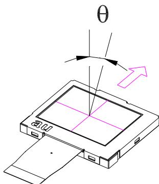
Note 8. Measure at the center area of the panel when all the input terminals of LCD panel are electrically opened.
