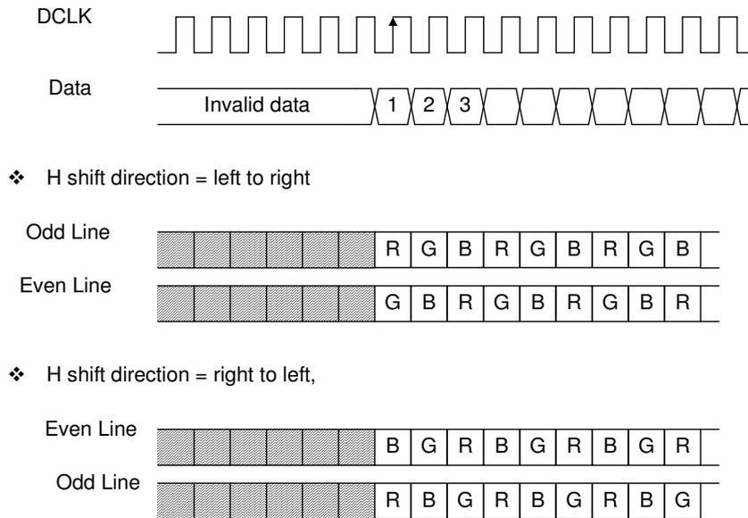
Fig. 10 UPS051 Input RGB sequence for 960x240 resolution
