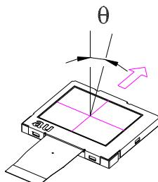
Note 8. Measured at the center area of the panel when all the input terminals of LCD panel are electrically opened
