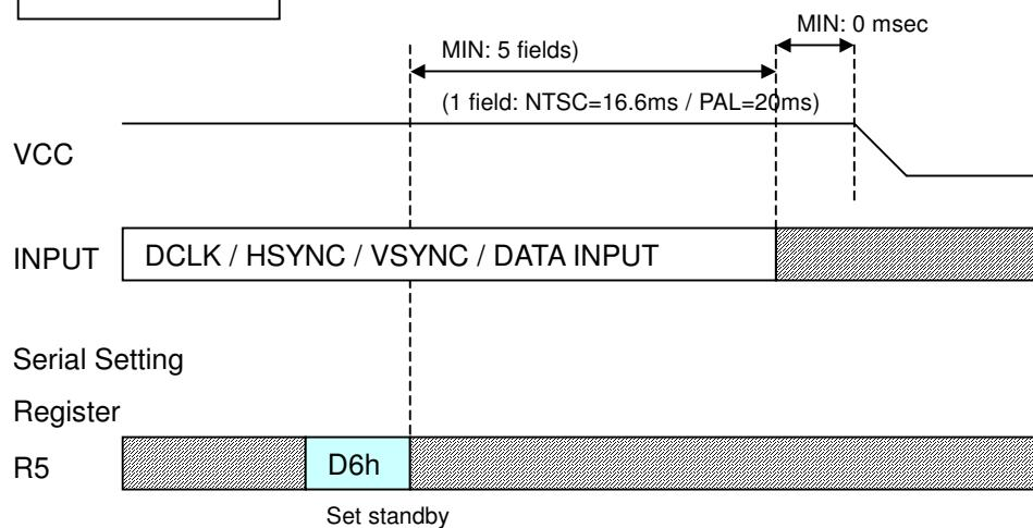
**Fig.16 Recommend serial command settings for UPS052 320x240**
