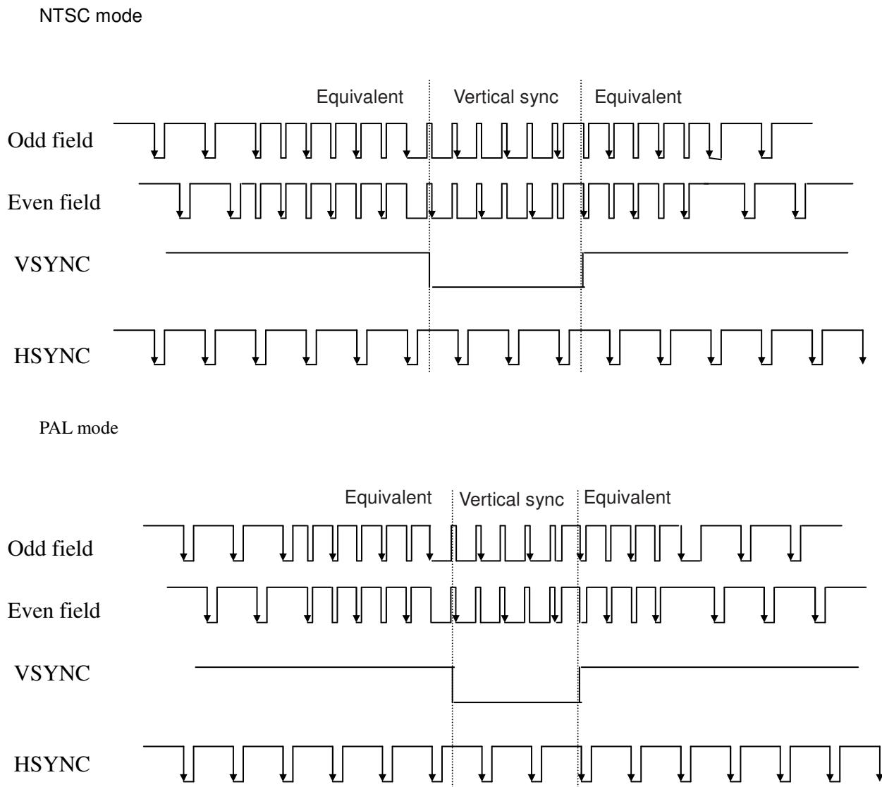
**Fig. 6: CSYNC Data input format**
