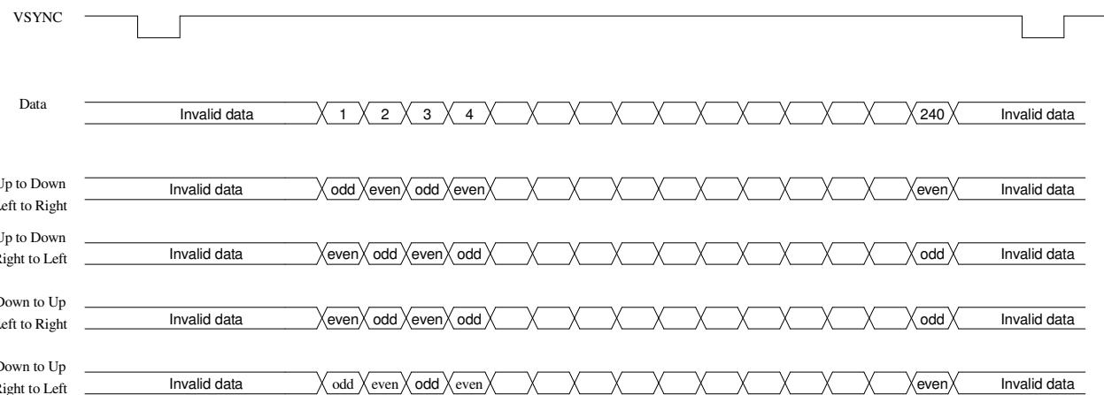
**Fig 9. UPS051 even and odd lines definition**
