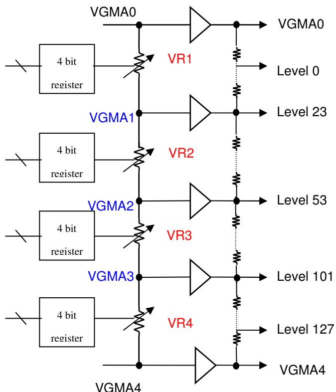
1. VGMA1, VGMA2, VGMA3 are generated within driver IC and adjustable through serial register setting
