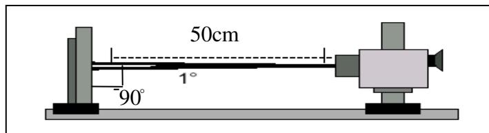
Note 4. Definition of response time: The output signals of photo detector are measured when the input signals are changed from "black" to "white"(falling time) and from "white" to "black"(rising time), respectively. The response time is defined as the time interval between the 10% and 90% of amplitudes. Refer to figure as below.
