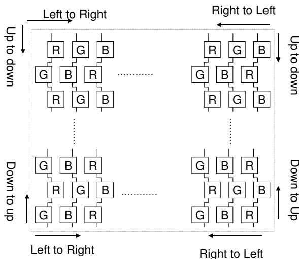
**Fig. 11 Color filter arrangement for 960x240 resolution**
