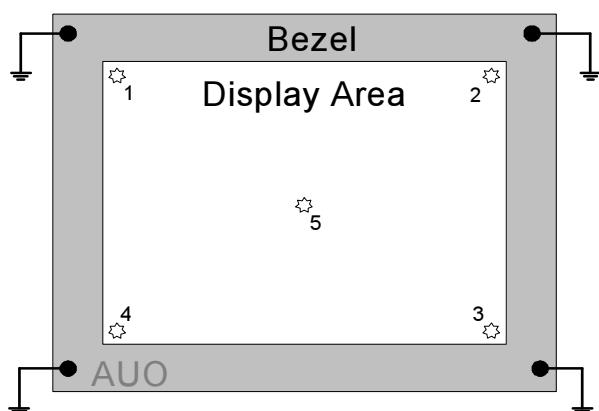
7. The metal casing is connected to power supply ground (0V) at four corners.
