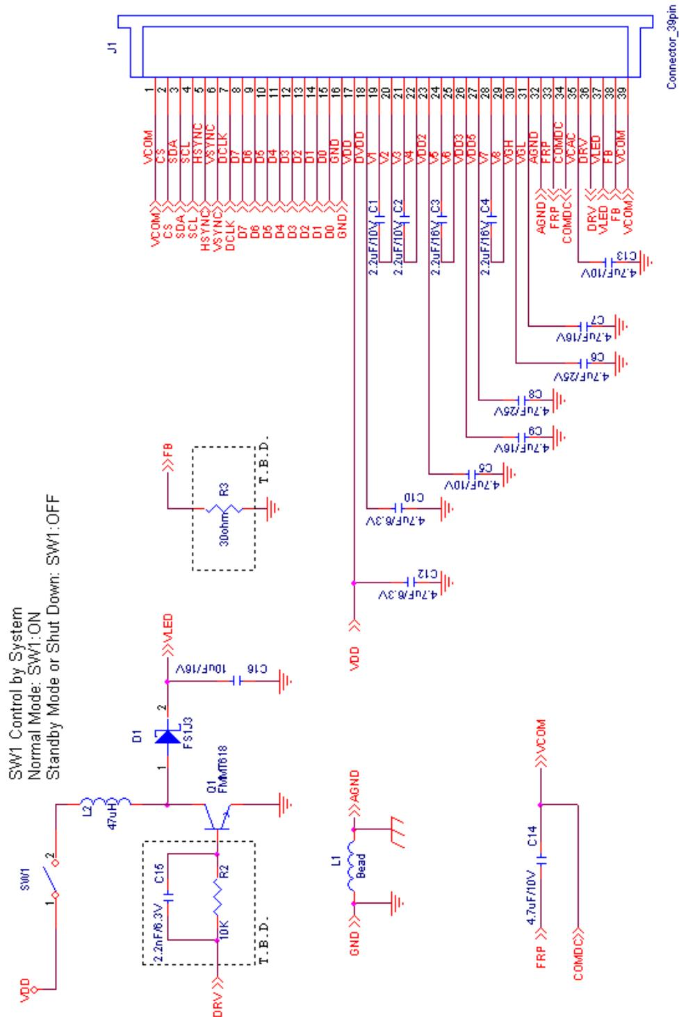
Note1: Use internal LED driver must set R5[1](SHDB1)= "1".
