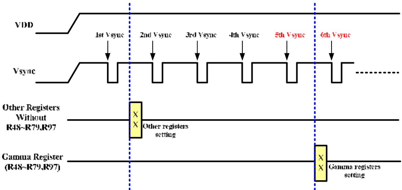
Note 1: Under different input timing, other registers setting please follow section "Recommended power on/off serial command settings".
