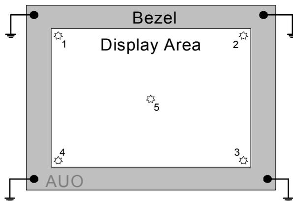
7. The metal casing is connected to power supply ground (0V) at four corners.
