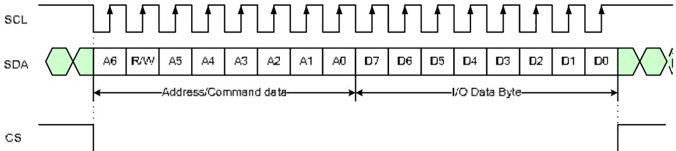
1. Each serial command consists of 16 bits of data which is loaded one bit a time at the rising edge of serial clock SCL.
