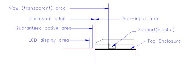
Do not put a heavy shock or stress on touch panel and film surface. Ex. Don't lift the panel by film face with vacuum.
