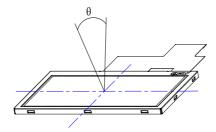
Note 9. Measured at the center area of the panel when all the input terminals of LCD panel are electrically opened.
