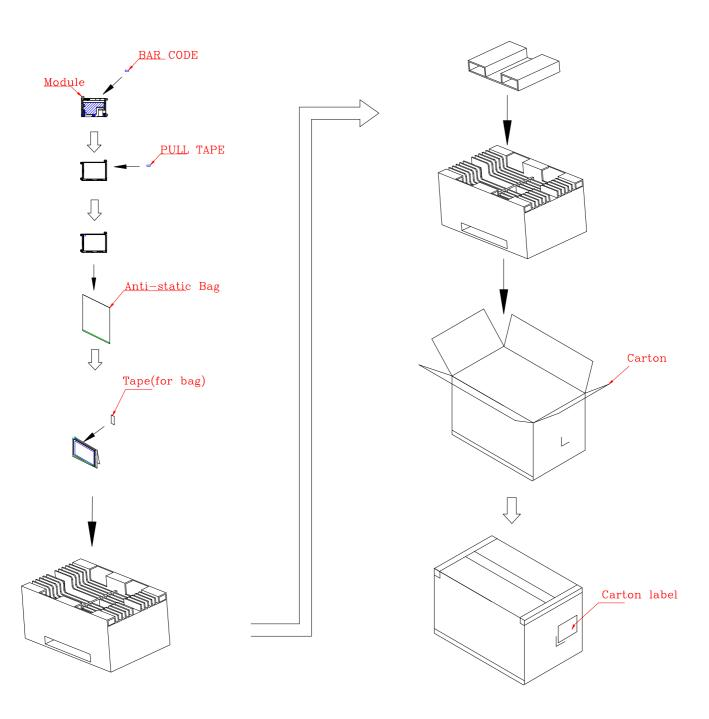
Max. Capacity: 40 Pcs Modules Max. Weight: 9.0 Kg Carton outline.: 520mm\*340mm\*250mm
