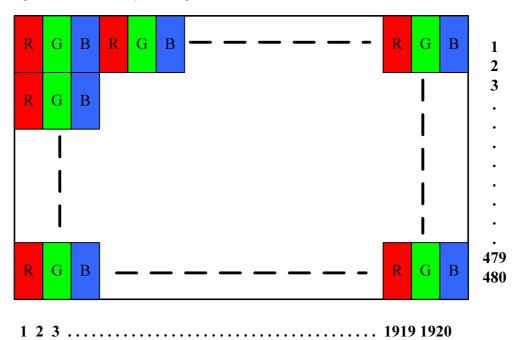
Note 2: Full color display depends on 6-bit data signal (pin 12~17, 19~24 and 26~31).
