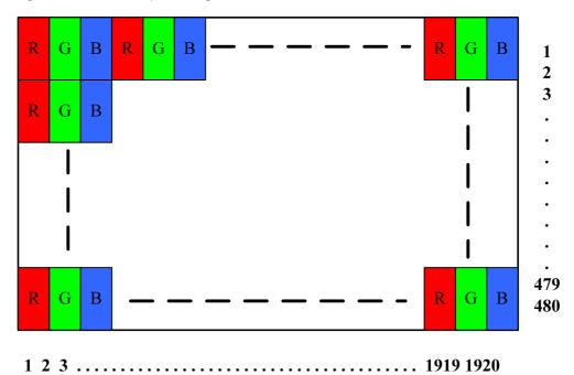
Note 2: Full color display depends on 6-bit data signal (pin 12~17, 19~24 and 26~31).
