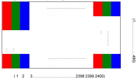
Note 3: The full color display depends on 24-bit data signal (pin 5~28).
