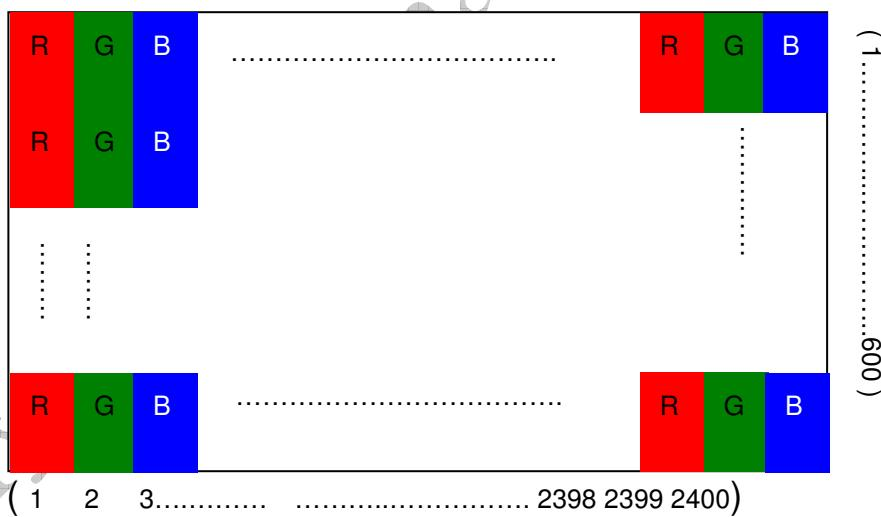
Note 3: The full color display depends on 24-bit data signal (pin 4~27).
