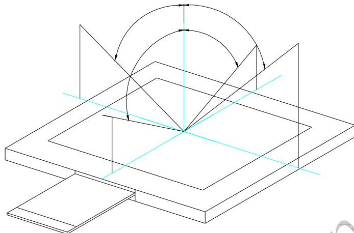
Note 6. Measured at the center area of the panel when all the input terminals of LCD panel are electrically opened.
