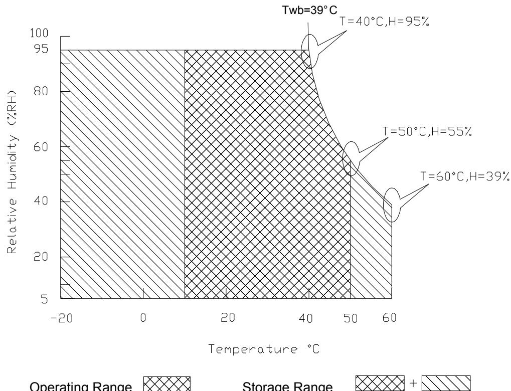
Note 2 : High Operating Temperature may cause the slight material variation. We assure under the above condition, the module set keep the function normal display.
