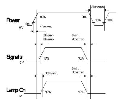
VDD power and lamp on/off sequence is as follows. Interface signals are also shown in the chart. Signals from any system shall be Hi-Z state or low level when VDD is off.
