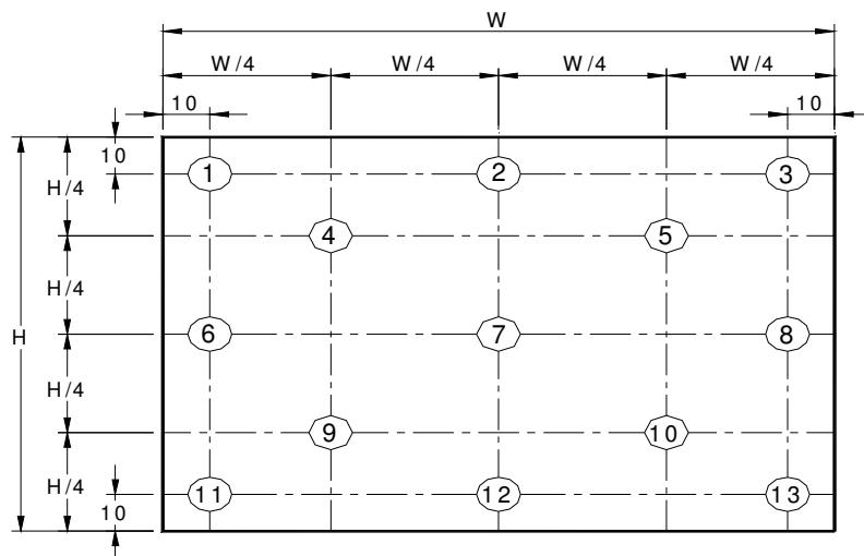
Note 3: The luminance uniformity of 13 points is defined by dividing the maximum luminance values by the minimum test point luminance
