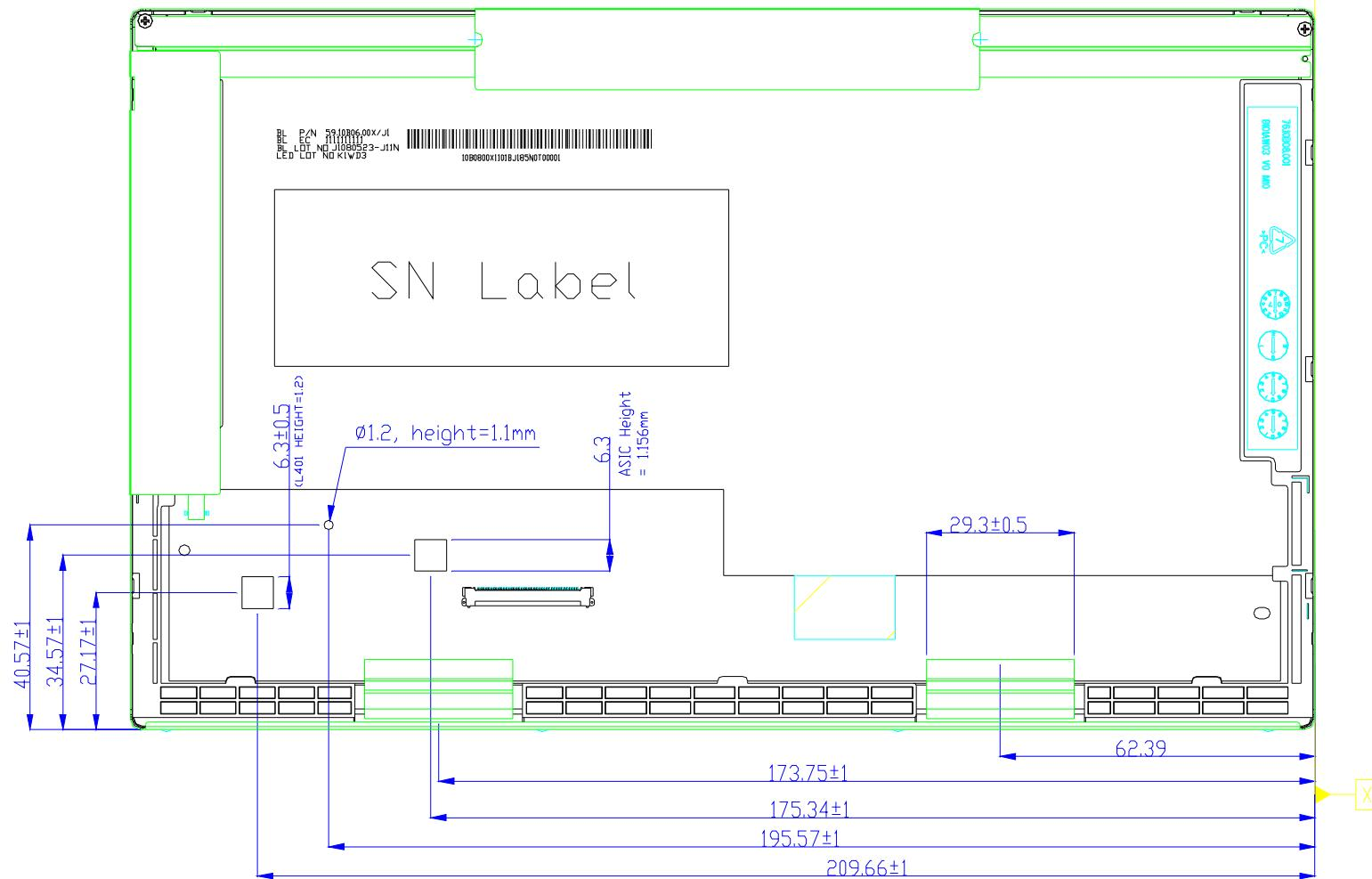
**11.2 Screw Hole Depth and Center Position:**
