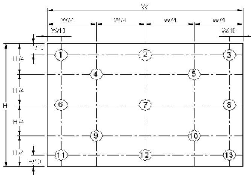
**Note 3:** The luminance uniformity of 5 and 13 points is defined by dividing the maximum luminance values by the minimum test point luminance
