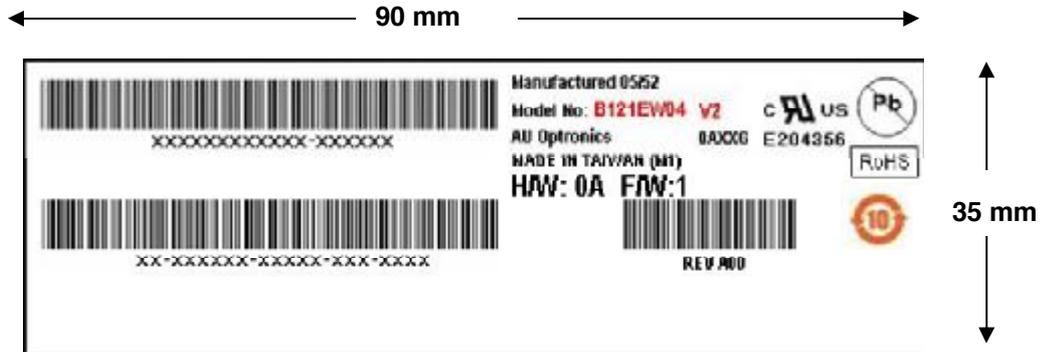
Carton label: This label is pasted on the carton to identify the quantity in each carton, Dell part number, and manufacture date.
