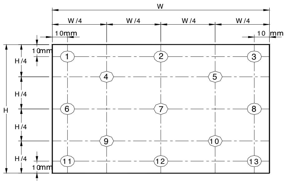
Note 3: The luminance uniformity of 5 or 13 points is defined by dividing the maximum luminance values by the minimum test point luminance. Length unit
