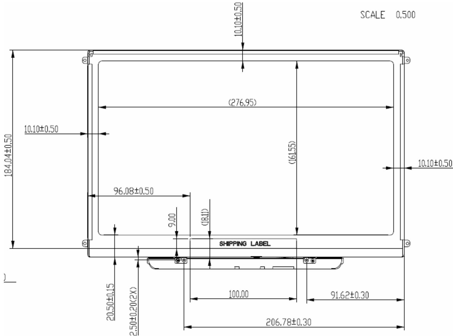
Note: Prevention IC damage, IC positions not allowed any overlap over these areas.
