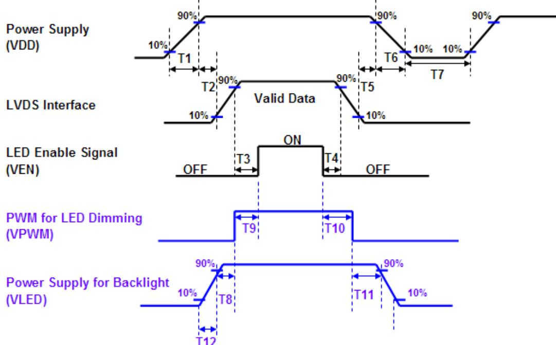
When the adapter is hot plugged, the backlight power supply sequence is shown as below.
