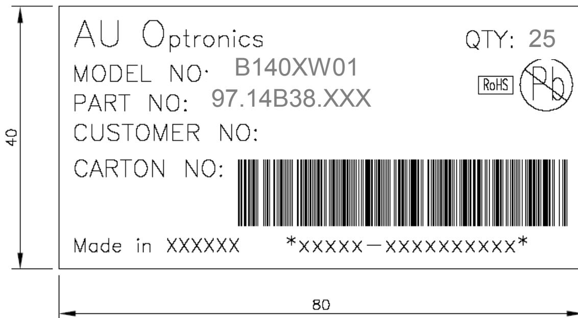
The outside dimension of carton is 454(L)mm\* 376(W)mm\* 302(H)mm, carton and cushion weight are 2200g
