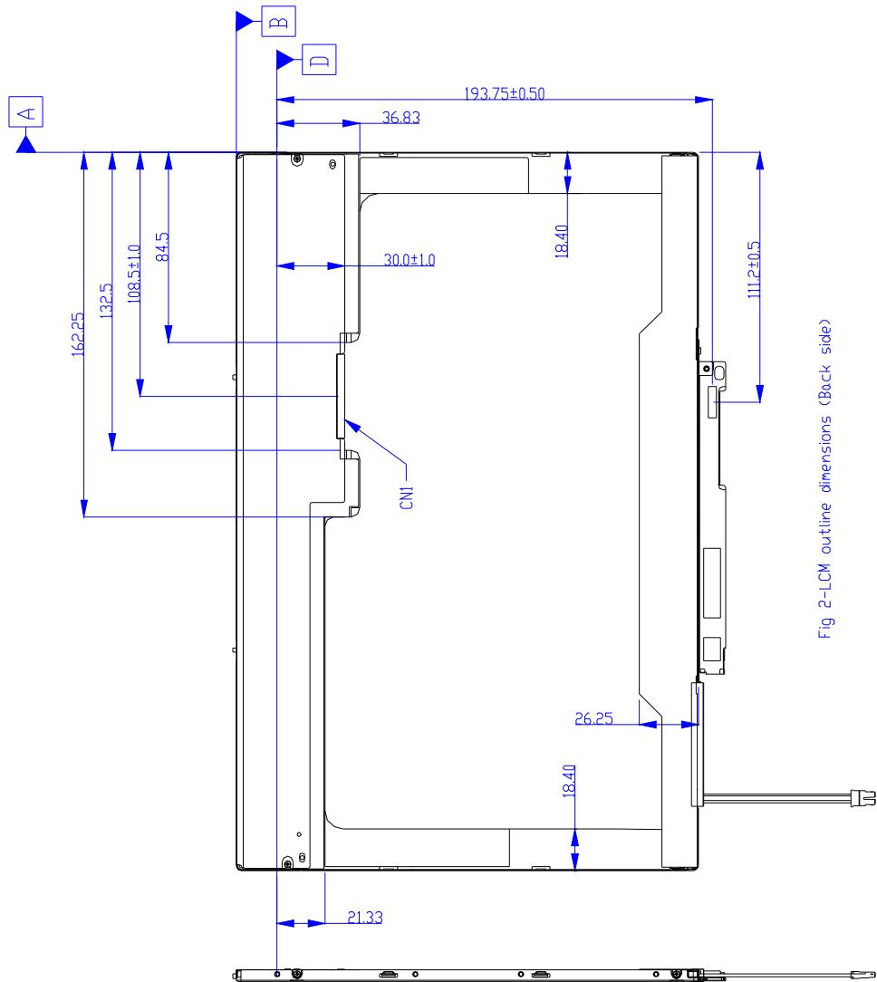
Fig 2-LCM outline dimensions (Back side)
