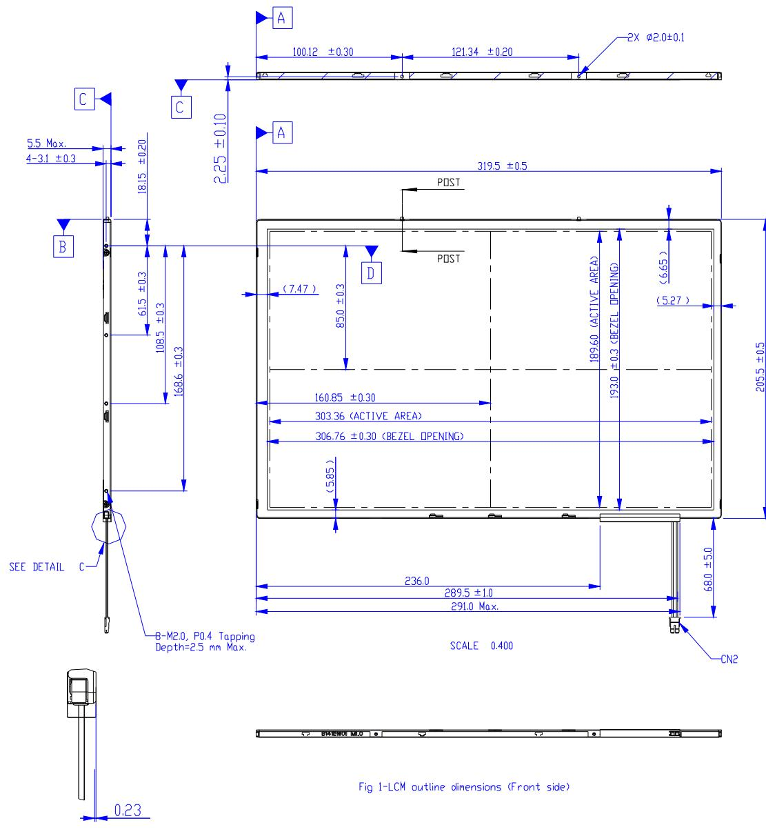
Fig 1-LCM outline dimensions (Front side)
