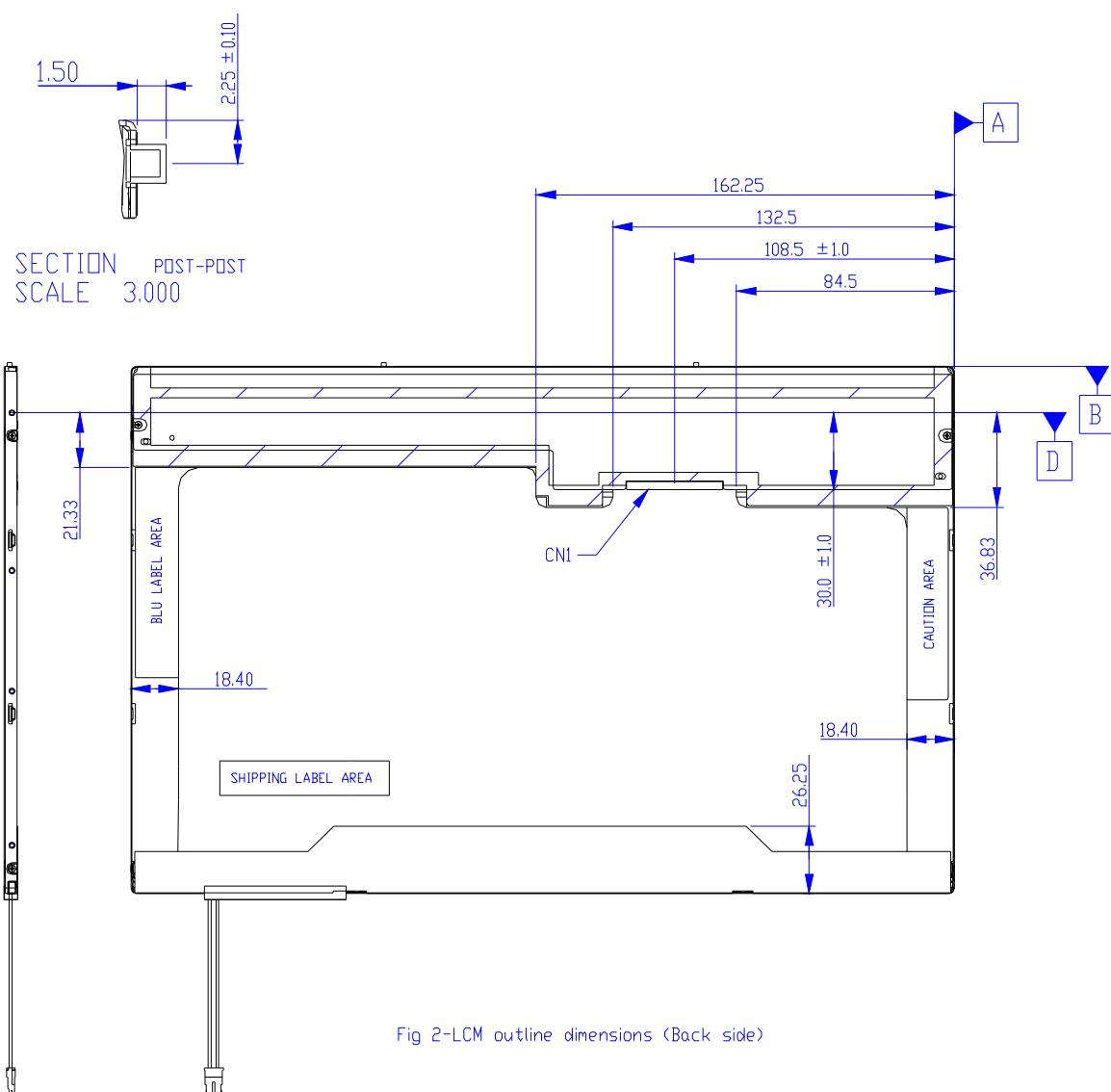
Fig 2-LCM outline dimensions (Back side)
