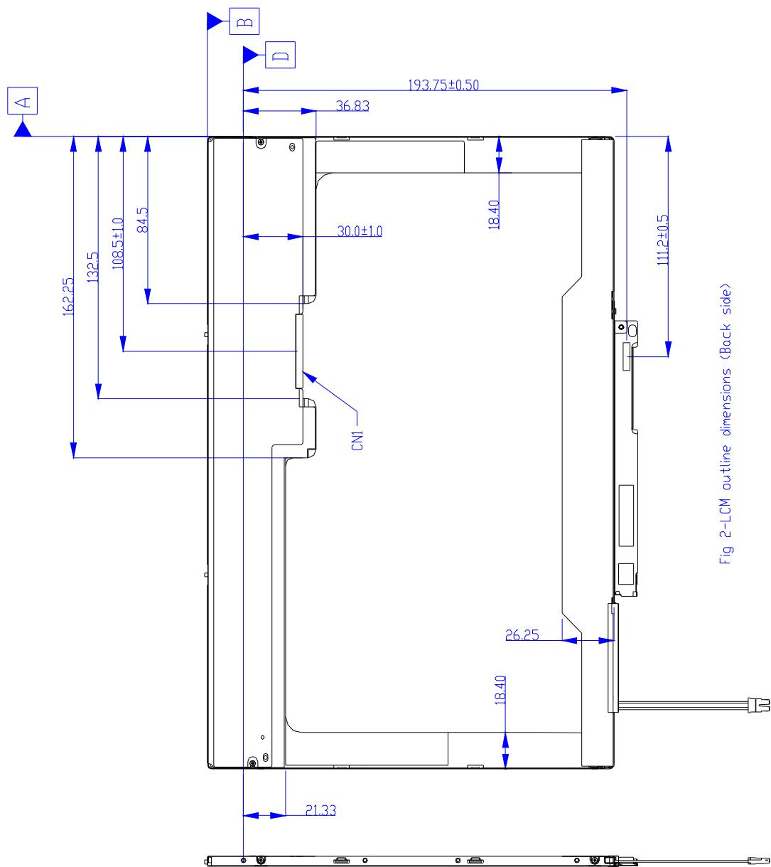
Fig 2-LCM outline dimensions (Back side)
