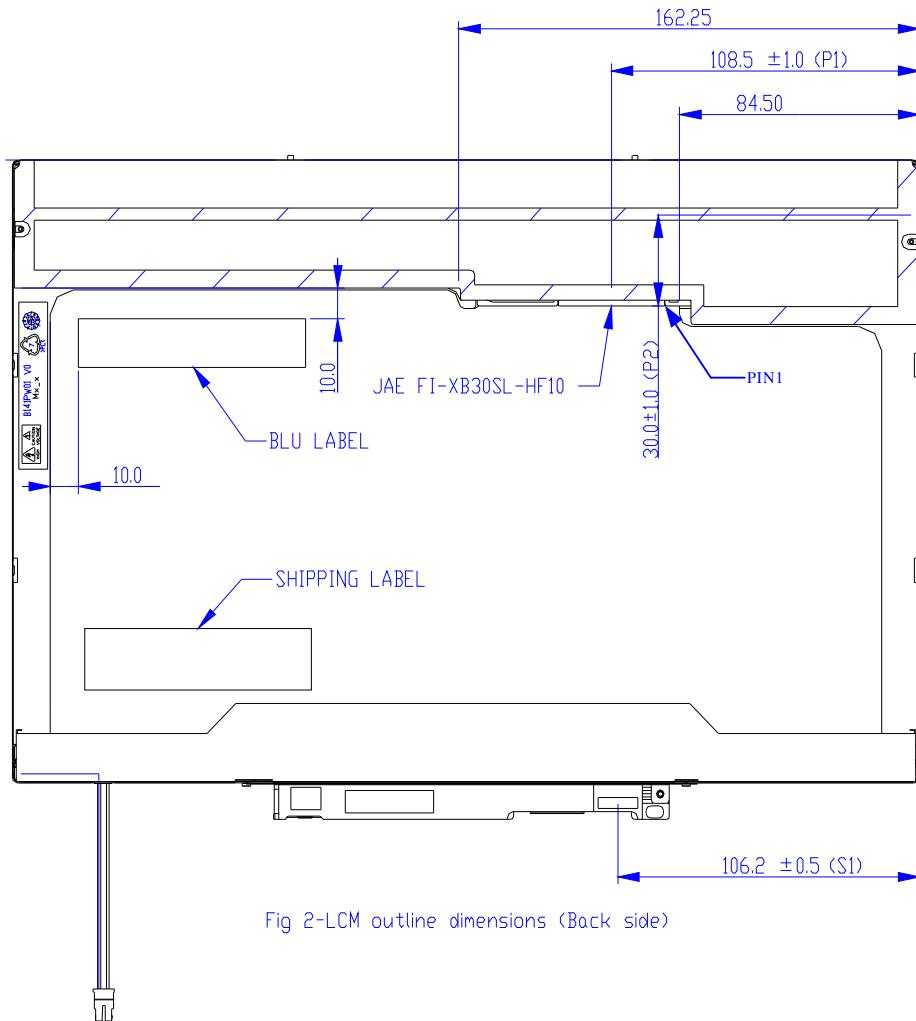
Fig 2-LCM outline dimensions (Back side)
