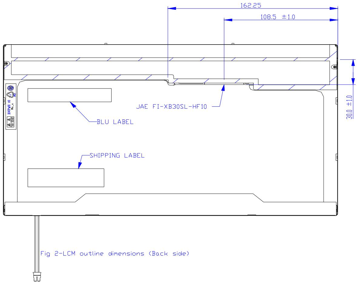
Fig 2-LCM outline dimensions (Back side)
