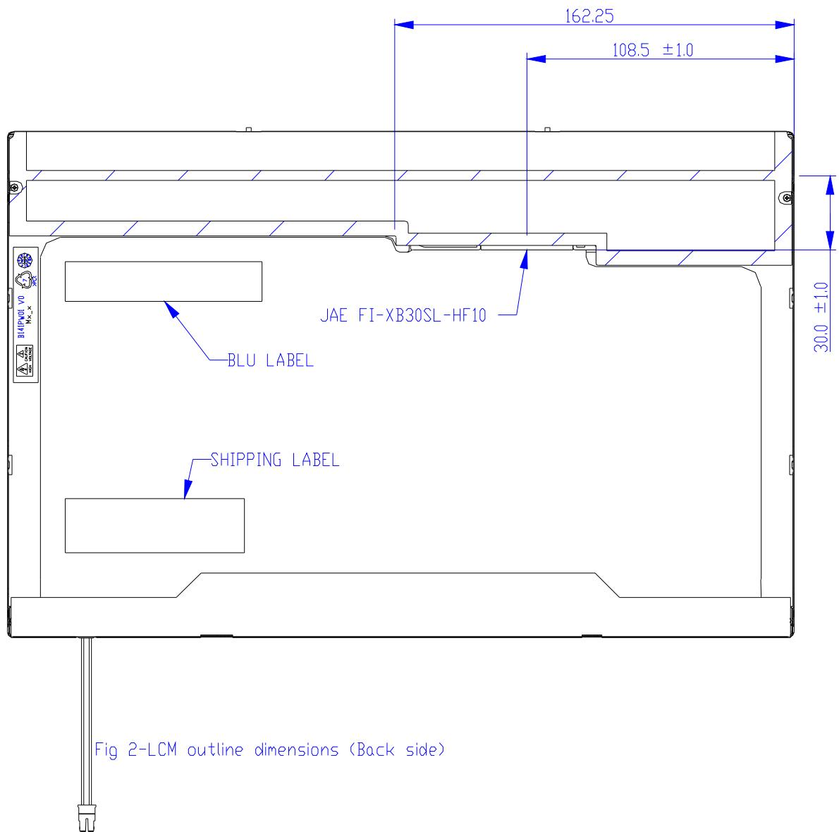
Fig 2-LCM outline dimensions (Back side)
