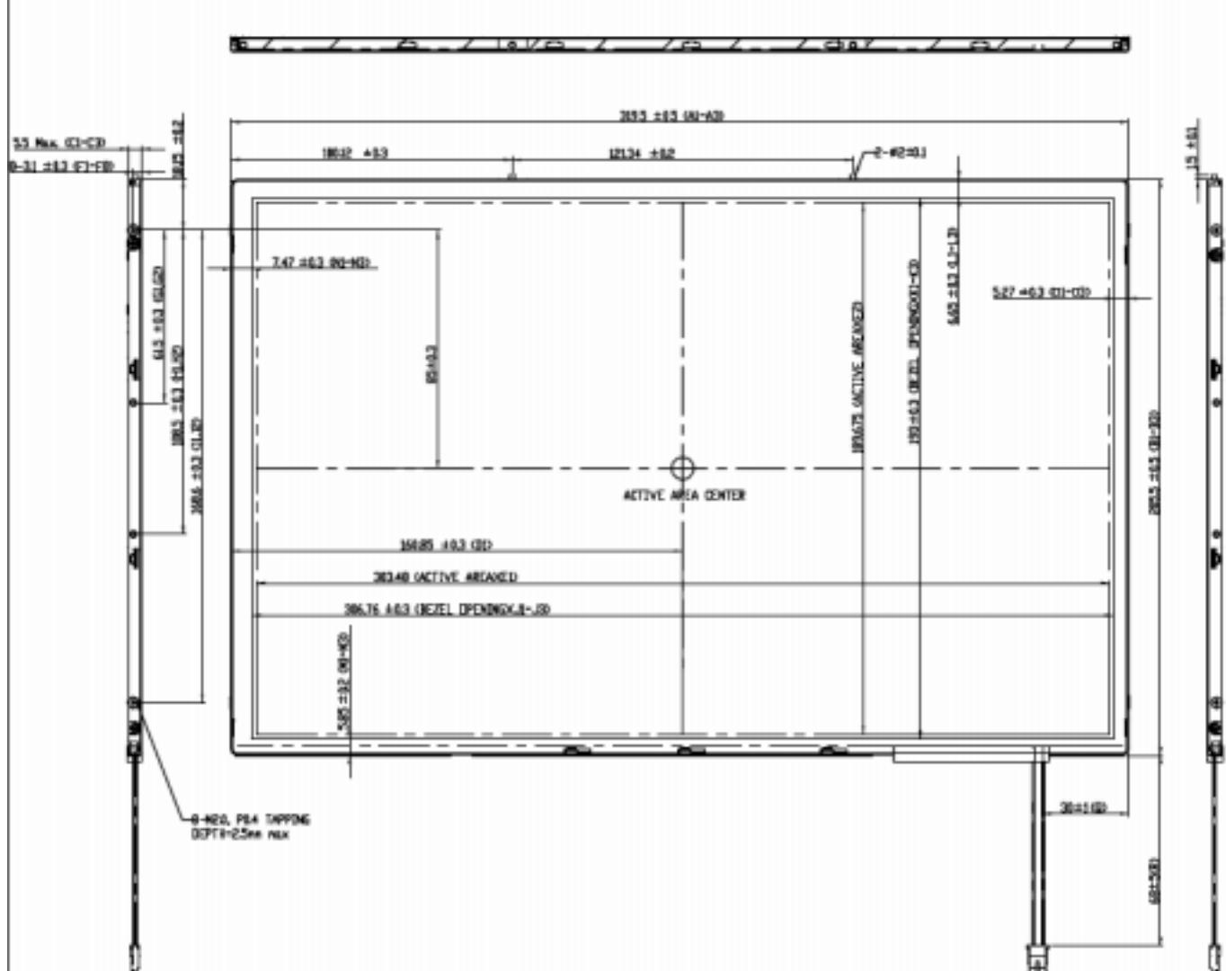
Fig 1-LCM outline dimensions (Front side)
