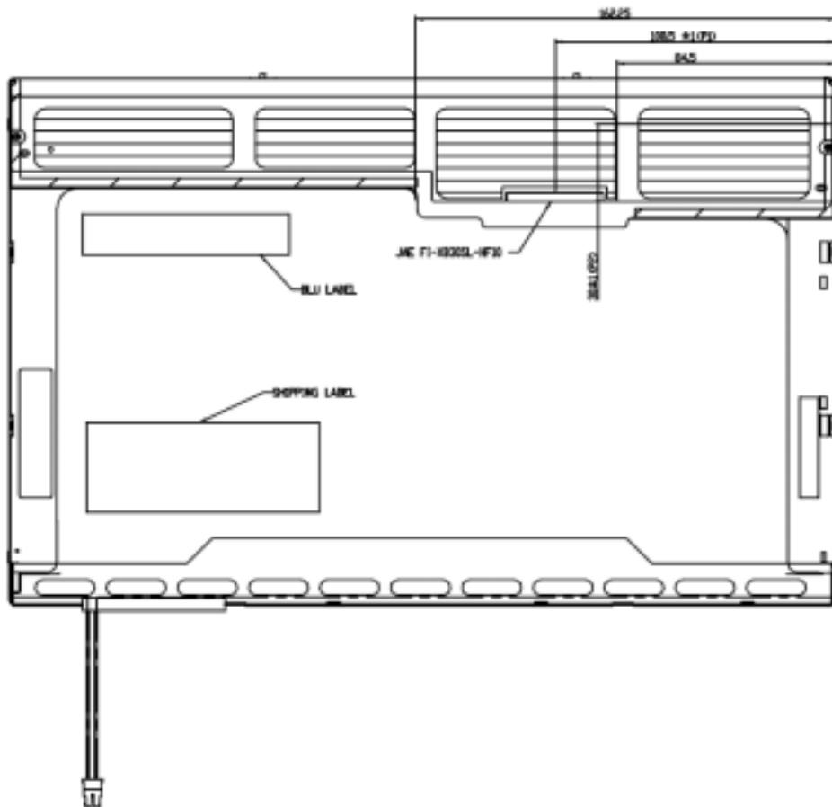
Fig. 2-LCD outline dimensions (Unit: mm)
