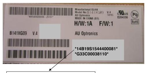
14B19 is Model Code S1 is Factory Code 544 is Manufacture Date (first digit is year code, 2<sup>nd</sup> & 3<sup>rd</sup> digit are week code) 4 is Reversion No. 00081 is Series Code.
