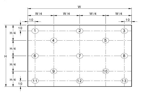
Note 3: The luminance uniformity of 5 and 13 points is defined by dividing the maximum luminance values by the minimum test point luminance
