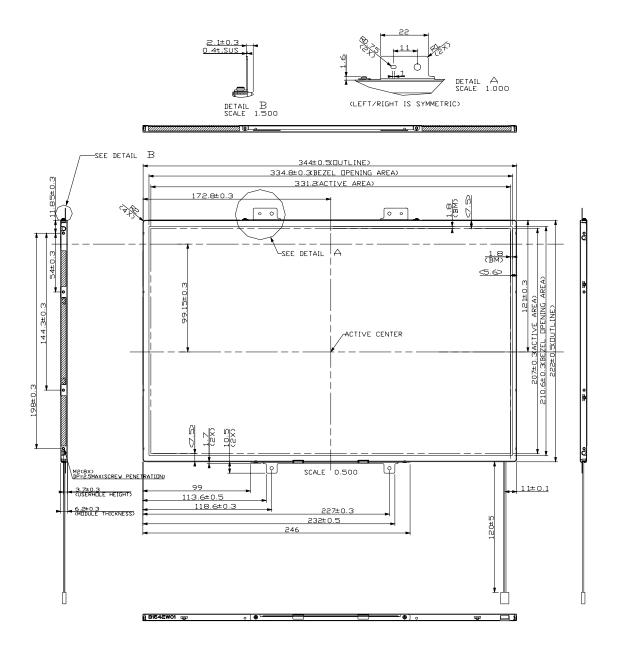
\* The screw hole depth is 2.5mm max
