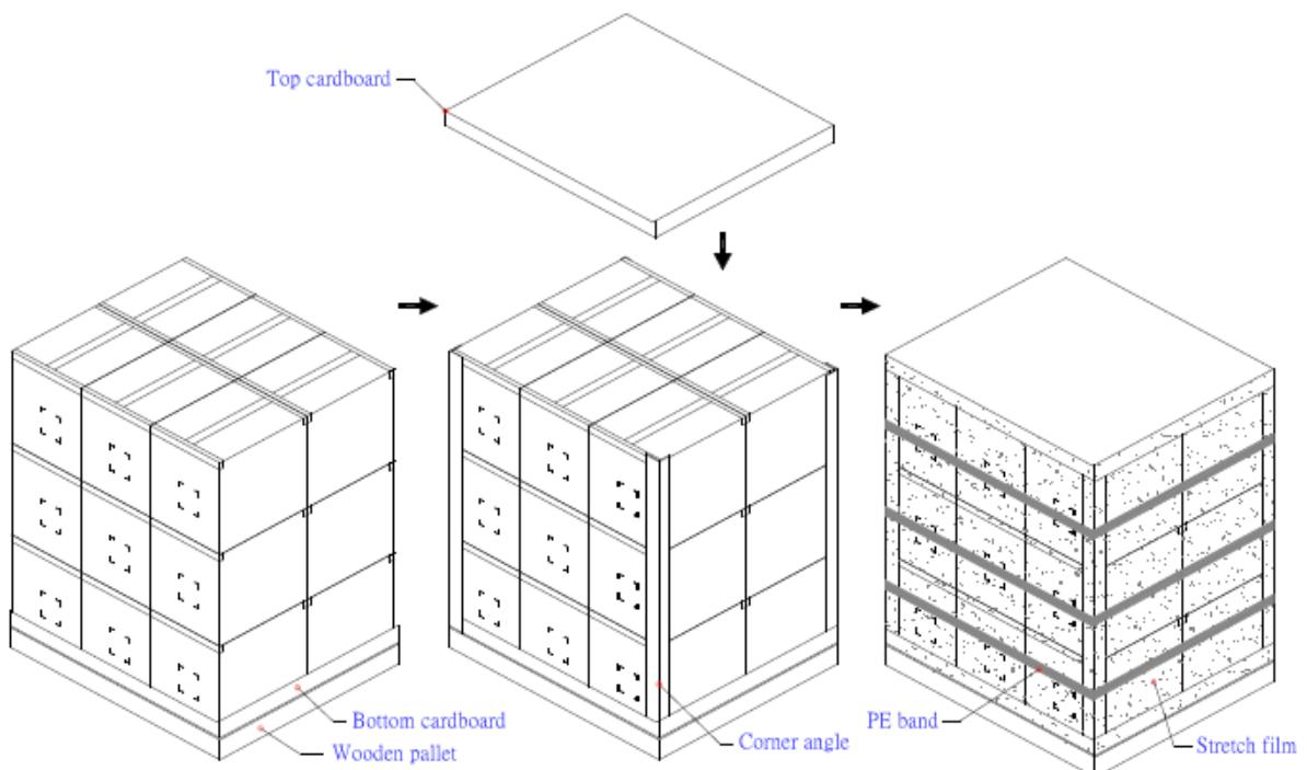
Note : Limit of box palletizing = Max 3 layers(ship and stock conditions)
