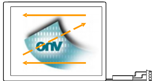
Fig. 2 Reverse scan (Pin31, DPS = High)
