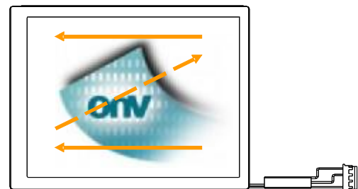
Fig. 2 Reverse scan (Pin4, DPS = High)
