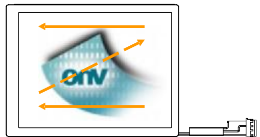
Fig. 2 Reverse scan (Pin4, DPS = High)
