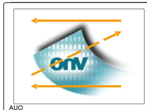
Fig. 1 Normal scan (Pin4, REV = Low or NC)
