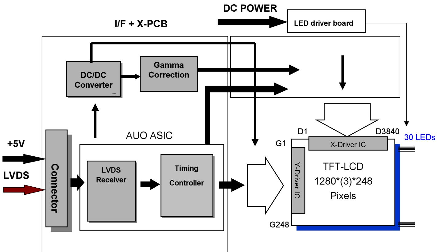
LVDS Connector: JAE (FI-XB30SSL-HF15) or equivalent.
