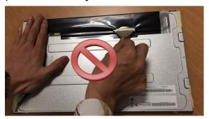
Do not insert the connector with single hand and touching the PCBA.
