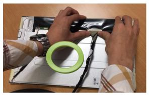
Insert the connector by pushing right and left edge.
