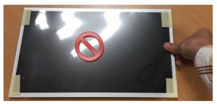
Do not press edge of panel to avoid glass broken.
