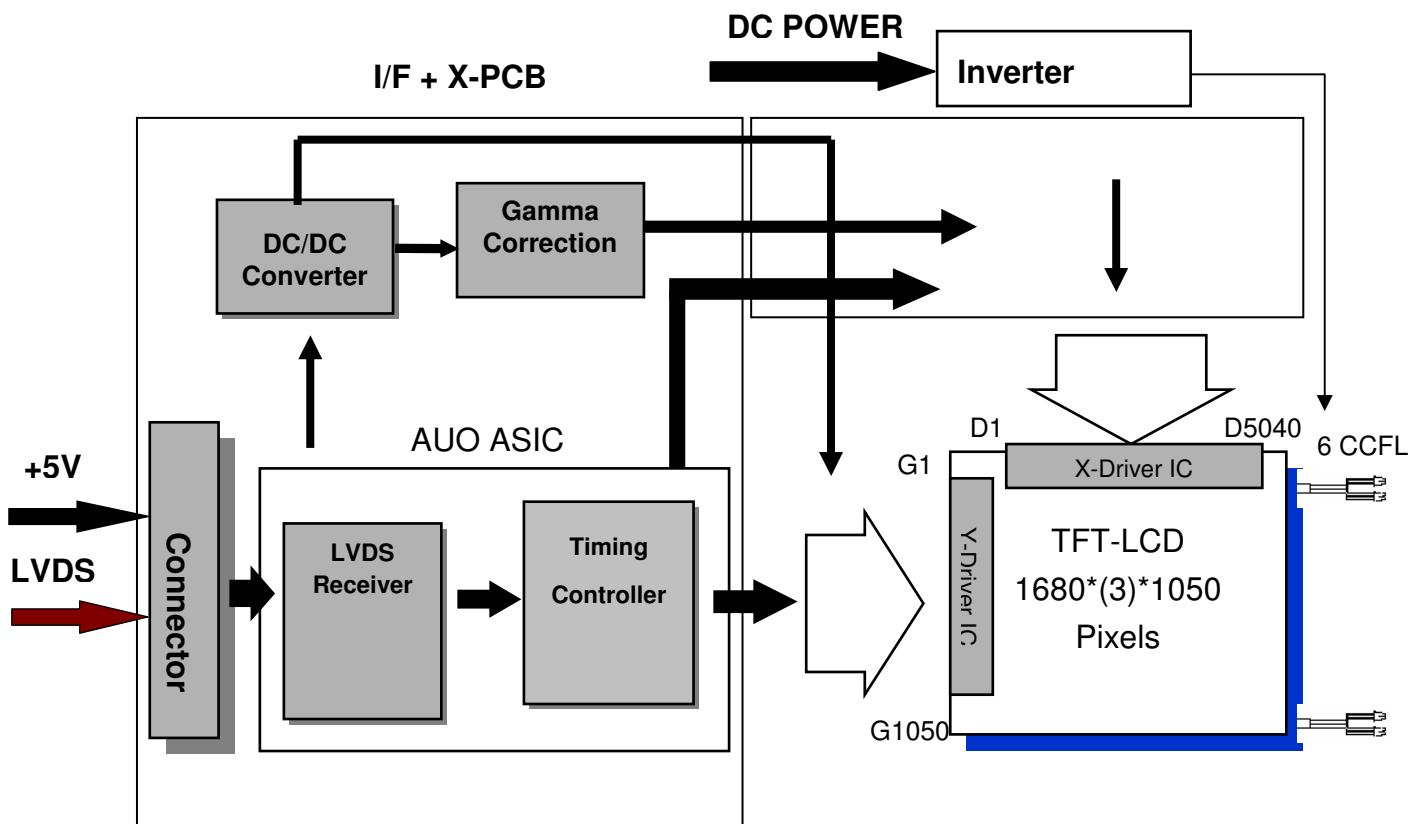
LVDS Connector: JAE (FI-XB30SRL-HF11) or equivalent.
