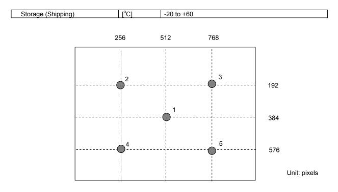
Note 1: Brightness is measured at the center point of brightness value with all pixels displaying white.
