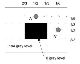
I  $L_A$ - $L_{A'}$  I /  $L_A$  x 100%= 1.2% max.,  $L_A$  and  $L_B$  are brightness at location A and B I  $L_B$ - $L_{B'}$  I /  $L_B$  x 100%= 1.2% max.,  $L_{A'}$  and  $L_{B'}$  are brightness at location A' and B'
