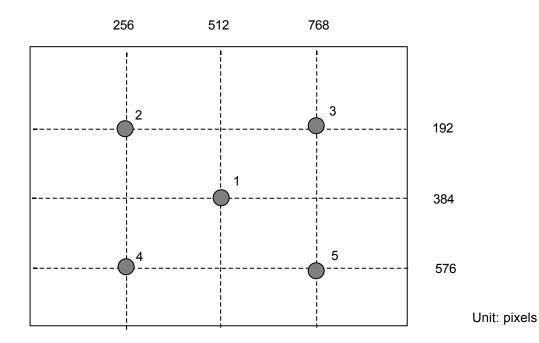
Note 1: Brightness is measured at the center point of brightness value with all pixels displaying white.
