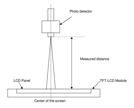
Note 2: Definition of viewing angle measured by ELDIM (EZContrast 88)
