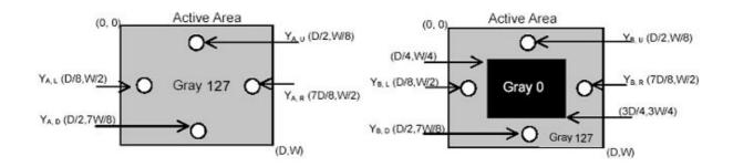
Note 9: Test Patern: Subchecker Pattern measured by TOPCON SR-3
