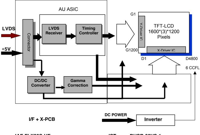
JAE FI-X30S-HF Mating Type: JAE FI-X30S-H JST BHSR-02VS-1 Mating Type: SM02B-BHSS-1-TB
