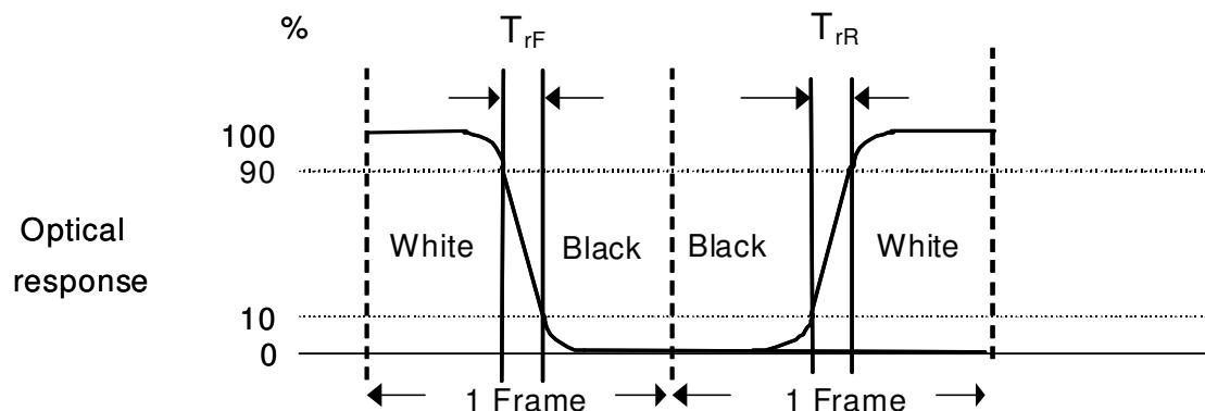
$$T_{rR} + T_{rF} = 25 \text{ msec (typ.)}$$
