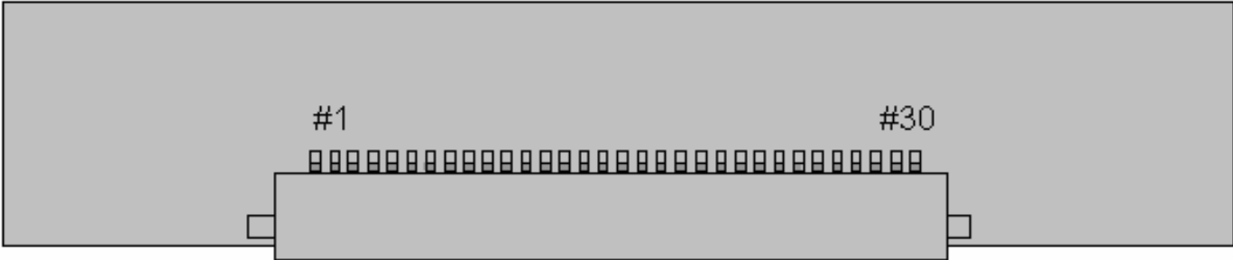
Top view of LVDS connector
