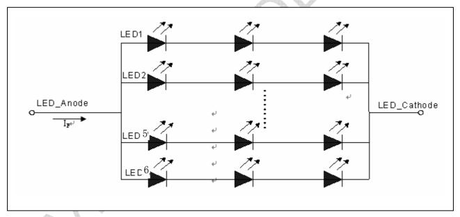
Note4: The LED driving condition is defined for each LED module.
