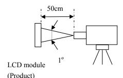
Luminance Meter (TOPCON BM-5A) Spectroradiometer (TOPCON SR-3)
